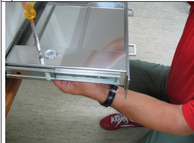
Unscrew both screws around sensor, holding the sensor under the drawer.
